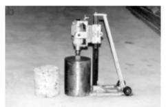
**Fig. 2:** A photograph of an air powered diamond coring machine used in replacing anchor bolts without regrouting the machinery.
