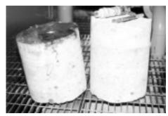
Fig. 3: A photograph of 12 inch dia. cores removed in the course of complete replacement of an anchor bolt. Note the cross section of a No. 11 rebar in the core.
