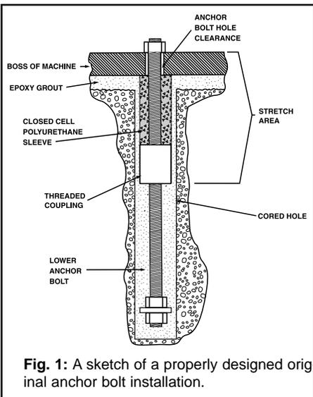
**Fig. 1:** A sketch of a properly designed original anchor bolt installation.
