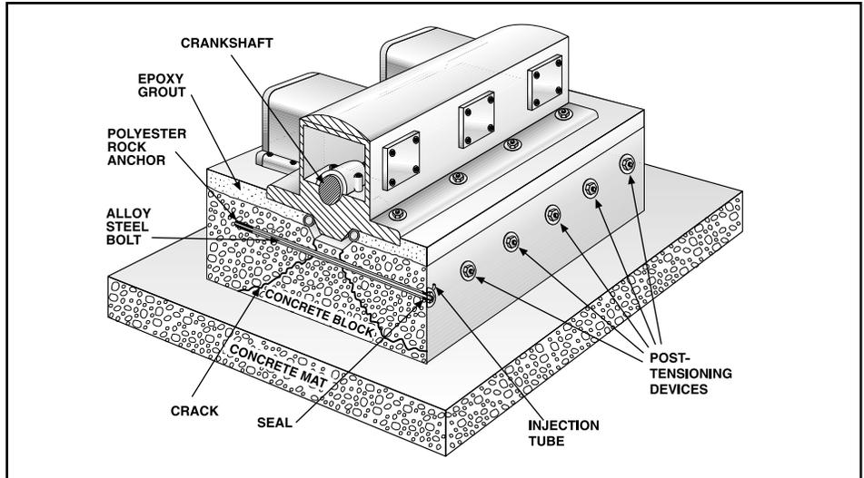
Fig. 1: Method of repairing compressor foundations that are cracked parallel to the crankshaft.
