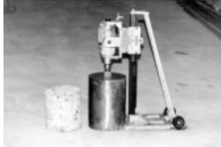
**Fig. 2:** A photograph of an air powered diamond coring machine used in replacing anchor bolts without regrouting the machinery.
