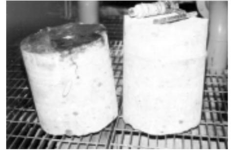
**Fig. 3:** A photograph of 12 inch dia. cores removed in the course of complete replacement of an anchor bolt. Note the cross section of a No. 11 rebar in the core.
