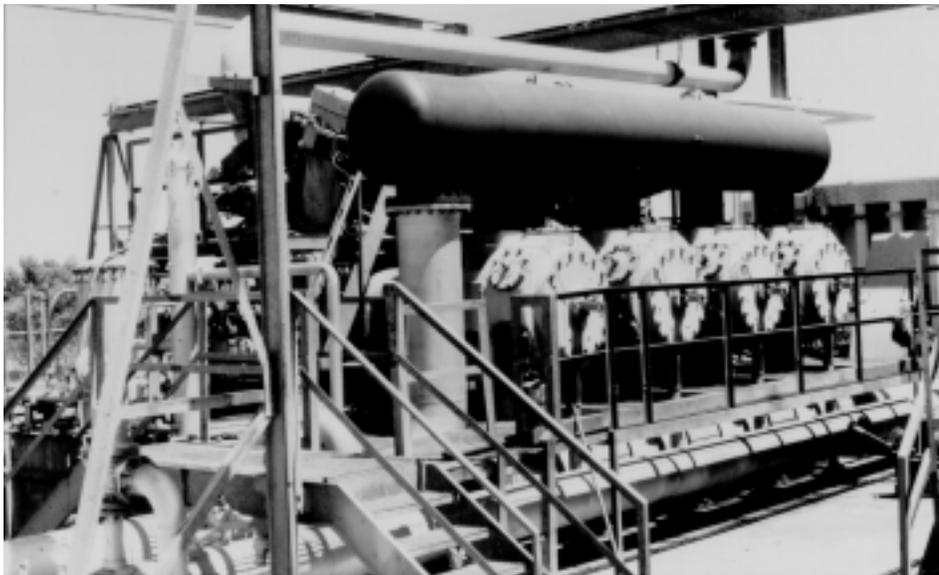
Fig. 1: A typical skid mounted integral gas engine compressor complete with accessories, controls and instrumentation.
